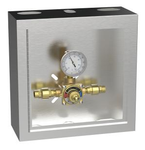
The Emergency Shower Mixing Valve shall employ a single control mechanism which split the flow in half, blend each half to the design temperature and then integrate each stream at the outlet. The valve shall control outlet temperature over a wide range of flow and shall be suitable for eye/eye face wash applications in order to comply with ANSI standard Z358.1. The valve shall include a single thermometer to measure the outlet temperature. Temperature adjustment shall be vandal-resistant.
