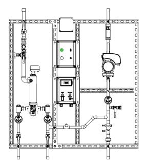
Mixing valve shall be incorporated into a completely assembled and tested pre-piped manifold system which includes a recirculating pump, circuit setting balancing valve, aquastat, circulator switch box, thermometers, ball valves, mounting strut, SEA Basic Digital System and test connection.
