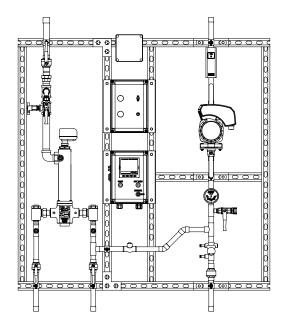
Mixing valve shall be incorporated into a completely assembled and tested pre-piped manifold system which includes a recirculating pump, circuit setting balancing valve, aquastat, circulator switch box, thermometers, ball valves, mounting strut, SEA Deluxe Digital System and test connection.
