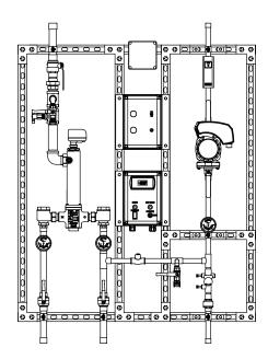
Mixing valve shall be incorporated into a completely assembled and tested pre-piped manifold system which includes a recirculating pump, circuit setting balancing valve, aquastat, circulator switch box, thermometers, ball valves, mounting strut, SEA Basic Digital System and test connection.
