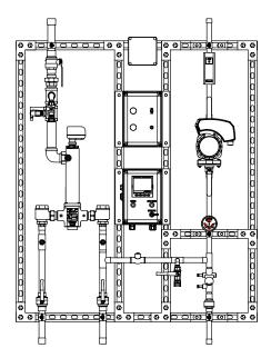
Mixing valve shall be incorporated into a completely assembled and tested pre-piped manifold system which includes a recirculating pump, circuit setting balancing valve, aquastat, circulator switch box, thermometers, ball valves, mounting strut, SEA Deluxe Digital System and test connection.
