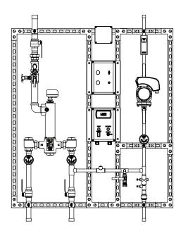
Mixing valve shall be incorporated into a completely assembled and tested pre-piped manifold system which includes a recirculating pump, circuit setting balancing valve, aquastat, circulator switch box, thermometers, ball valves, mounting strut, SEA Basic Digital System and test connection.
