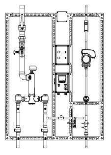
Mixing valve shall be incorporated into a completely assembled and tested pre-piped manifold system which includes a recirculating pump, circuit setting balancing valve, aquastat, circulator switch box, thermometers, ball valves, mounting strut, SEA Deluxe Digital System and test connection.
