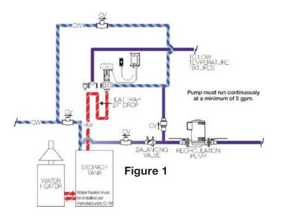
When installing the Lawler Neptune EMX Electronic Mixing valve into a single temperature recirculating system, please install as shown in Figure 1.
