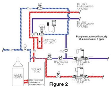
When installing the Lawler Neptune EMX Electronic Mixing Valve into a dual temperature recirculating system, please install as shown in Figure 2.
