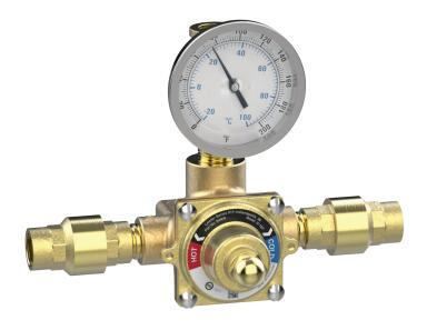
The Emergency Shower Mixing Valve shall employ a single control mechanism which split the flow in half, blend each half to the design temperature and then integrate each stream at the outlet. The valve shall control outlet temperature over a wide range of flow and shall be suitable for eye/eye face wash applications in order to comply with ANSI standard Z358.1. The valve shall include a single thermometer to measure the outlet temperature. Temperature adjustment shall be vandal-resistant.
