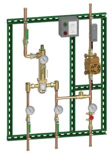
Mixing valve shall be incorporated into a completely assembled and tested pre-piped manifold system which includes a recirculating pump, circuit setting balancing valve, aquastat, circulator switch box, thermometers, ball valves, mounting strut, and test connection.
