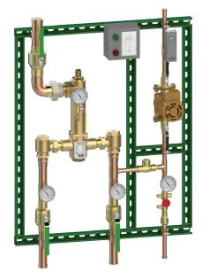
Mixing valve shall be incorporated into a completely assembled and tested pre-piped manifold system which includes a recirculating pump, circuit setting balancing valve, aquastat, circulator switch box, thermometers, ball valves, mounting strut, and test connection.
