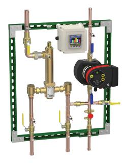
Mixing valve shall be incorporated into a completely assembled and tested pre-piped manifold system which includes a Grundfos Magna3 32-60 F N pump, circuit setting balancing valve, thermometers, ball valves, mounting strut, and test connection.
