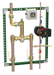
Mixing valve shall be incorporated into a completely assembled and tested pre-piped manifold system which includes a Grundfos Magna3 32-60 F N pump, circuit setting balancing valve, thermometers, ball valves, mounting strut, and test connection.
